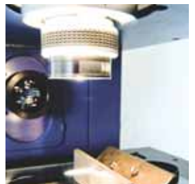
Inspection by the profile projector: it is used to measure the dimensional contours and areas which are inaccessible to conventional measuring devices
