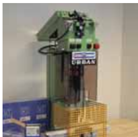
Application test: a bolt is screwed into the window frame by a reinforcement screwing unit Urban
