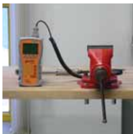
Measuring of torque strength: a torque wrench and digital evaluation unit are used to measure the torque, and the maximum value is also recorded
