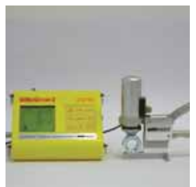
Hardness test: variable portable hardness measuring device is used to measure the hardness of the material
