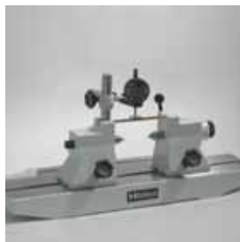
Inspection of the circular runout: measuring the straightness of bolts
