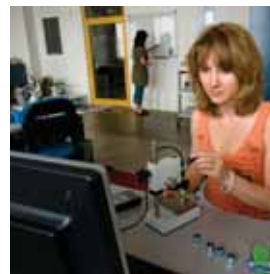
Measuring of the surface layer thickness: the thickness of the surface layer is measured by a probe and the evaluation unit
