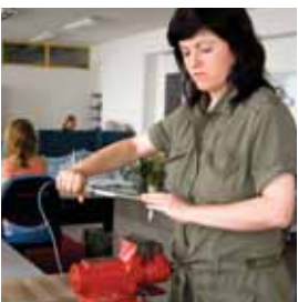
Measuring of torque strength: a torque wrench and digital evaluation unit are used to measure the torque, and the maximum value is also recorded
