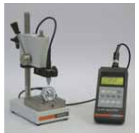
Measuring of the surface layer thickness: the thickness of the surface layer is measured by a probe and the evaluation unit
